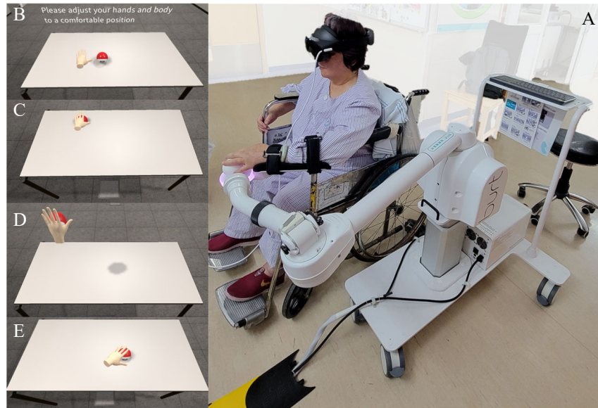
Fig. 1. Overview of the study: (A) The participant wears the BURT and the VR headset. BURT helps participants cancel out the burden of gravity on the affected arm. (B) Warm-up for VR Rehabilitation scene with text hint: “Please adjust your hands and body to a comfortable position” (C) The participant performs reaching in VR, corresponding to depth; (D) The participant performs shoulder flexion in VR, corresponding to vertical; (E) The participant performs horizontal abduction in VR, corresponding to horizontal.
